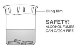
6. After 24 hours, remove the chips from the alcohol and the beaker.
