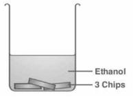
5. Ensure the chips are fully submerged, and cover the beaker tightly with cling film.
